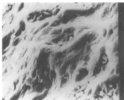
FIGURE 9 SEM Photograph (800X) of LLDPE/CSM (60/40) R-T stretched sample.
